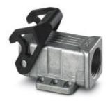
Box mounting bases D7, With single locking latch, Material: Die-cast aluminum, salt water resistant, Cable outlets: 1, lateral, Height: 27.9 mm, Cable gland: none, Gland: no, 1x M20, Standard, enclosed bottom
