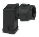
Sleeve housing D7, for single locking latch, Material: PA, Cable outlets: 1, lateral, Height: 54.5 mm, Cable gland: with, Gland: no, 1x M20, Standard
