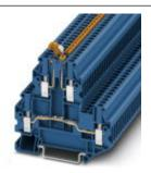
Knife disconnect terminal block, With test socket screws for insertion of test plugs, Connection type: Screw connection, Cross section: 0.14 mm² - 4 mm², AWG: 26 - 12, Width: 5.2 mm, Color: blue, Mounting type: NS 35/7,5, NS 35/15
