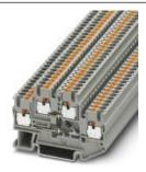
Component terminal block, with integrated diode, Connection type: Push-in connection, Cross section: 0.14 mm² - 4 mm², AWG: 26 - 12, Nominal current: 20 A, Nominal voltage: 500 V, Length: 68 mm, Width: 5.2 mm, Color: gray, Assembly: NS 35/7,5, NS 35/15
