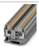
Feed-through terminal block, Connection method: Push-in connection, Cross section: 0.5 mm<sup>2</sup> - 10 mm<sup>2</sup>, AWG: 20 - 8, Width: 8.2 mm, Height: 42.2 mm, Color: orange, Mounting type: NS 35/7,5, NS 35/15
