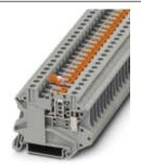
Knife disconnect terminal block, With test socket screws for insertion of test plugs, Connection type: Screw connection, Cross section: 0.14 mm² - 6 mm², AWG: 26 - 10, Nominal current: 20 A, Nominal voltage: 500 V, Length: 57.8 mm, Width: 6.2 mm, Color: orange, Assembly: NS 35/7,5, NS 35/15
