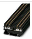
Feed-through terminal block, Connection method: Push-in connection, Cross section: 0.14 mm<sup>2</sup> - 1.5 mm<sup>2</sup>, AWG: 26 - 16, Width: 3.5 mm, Height: 30.5 mm, Color: black, Mounting type: NS 35/7,5, NS 35/15
