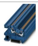
Installation terminal block, Push-in connection, Cross section: 0.14 mm² - 4 mm², AWG: 26 - 12, Width: 5.2 mm, Color: blue, Mounting type: NS 35/7,5, NS 35/15
