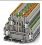
Knife disconnect terminal block, Connection type: Screw connection, Cross section: 0.14 mm² - 4 mm², AWG: 26 - 12, Nominal current: 16 A, Nominal voltage: 400 V, Length: 80.1 mm, Width: 5.2 mm, Color: gray, Assembly: NS 35/7,5, NS 35/15
