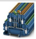
Knife disconnect terminal block, With test socket screws for insertion of test plugs, Connection type: Screw connection, Cross section: 0.14 mm² - 4 mm², AWG: 26 - 12, Nominal current: 16 A, Nominal voltage: 400 V, Length: 80.1 mm, Width: 5.2 mm, Color: blue, Assembly: NS 35/7,5, NS 35/15
