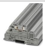
Installation level terminal block, Screw connection, Cross section: 0.2 mm² - 4 mm², AWG: 24 - 12, Width: 5.2 mm, Color: gray, Mounting type: NS 35/7,5, NS 35/15
