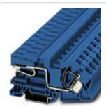
N disconnect terminal block, Spring-cage connection, Cross section: 0.2 mm² - 25 mm², AWG: 24 - 4, Width: 12 mm, Color: blue, Mounting type: NS 35/15, NS 35/7,5
