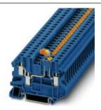
Knife disconnect terminal block, With test socket screws for insertion of test plugs, Connection type: Screw connection, Cross section: 0.14 mm² - 6 mm², AWG: 26 - 10, Nominal current: 20 A, Nominal voltage: 500 V, Length: 65.4 mm, Width: 6.2 mm, Color: blue, Assembly: NS 35/7,5, NS 35/15
