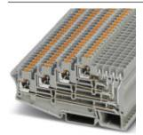
Multi-level terminal block, Connection method: Push-in connection, Cross section: 0.14 mm<sup>2</sup> - 4 mm<sup>2</sup>, AWG: 26 - 12, Width: 5.2 mm, Color: gray, Mounting type: NS 35/7,5, NS 35/15
