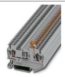
Knife disconnect terminal block, Connection type: Spring-cage connection, Cross section: 0.08 mm² - 4 mm², AWG: 28 - 12, Nominal current: 20 A, Nominal voltage: 400 V, Length: 60.5 mm, Width: 5.2 mm, Color: orange, Assembly: NS 35/7,5, NS 35/15
