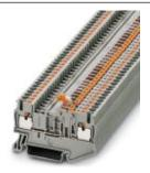
Knife disconnect terminal block, Connection type: Push-in connection, Cross section: 0.14 mm² - 4 mm², AWG: 26 - 12, Nominal current: 20 A, Nominal voltage: 400 V, Length: 62 mm, Width: 5.2 mm, Color: orange, Assembly: NS 35/7,5, NS 35/15
