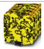
High-current terminal block, Connection method: Power-Turn connection, Cross section: 25 mm<sup>2</sup> - 95 mm<sup>2</sup>, AWG: 4 - 3/0, Width: 25 mm, Height: 99.8 mm, Color: black/yellow, Mounting type: NS 35/15
