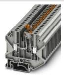
Knife disconnect terminal block, With test socket screws for insertion of test plugs, Connection type: Screw connection with spring support, Cross section: 0.2 mm² - 6 mm², AWG: 24 - 10, Nominal current: 20 A, Nominal voltage: 500 V, Length: 63.4 mm, Width: 6.2 mm, Color: gray, Assembly: NS 35/7,5, NS 35/15, NS 32
