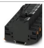
Fuse modular terminal block, Connection method: Push-in connection, Cross section: 1.5 mm²- 10 mm², AWG: 16 - 6, Nominal current: 20 A, Nominal voltage: 1000 V, Width: 17.6 mm, Fuse type: Midget / 10.3 x 38, Mounting type: NS 35/7,5, NS 35/15, Color: black
