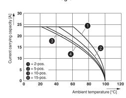
The figure shows the derating curve of the UT 2,5/1P... terminal block in connection with the UPBV 2,5 plug
