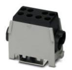
Trunk line branch terminal, Connection method: Screw connection, Screw connection, Number of positions: 1, Cross section: 10 mm² - 35 mm², AWG: 8 - 2, Width: 27 mm, Color: black, Mounting type: NS 35/7,5, NS 35/15
