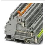
Ground modular terminal block, Connection type: Screw connection, Cross section: 0.14 mm² - 6 mm², AWG: 26 - 10, Nominal current: 28 A, Nominal voltage: 500 V, Length: 92.7 mm, Width: 6.2 mm, Color: gray, Assembly: NS 35/7,5, NS 35/15
