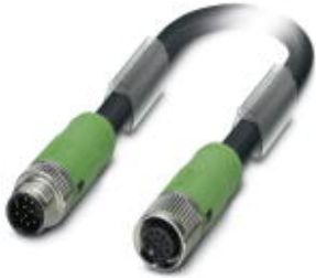
Sensor/Actuator cable, 12-position, PUR/PVC, black RAL 9005, shielded, Plug straight M12 SPEEDCON, A-coded, on Socket straight M12 SPEEDCON, A-coded, Cable length: 3 m
