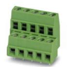
PCB terminal block, Nominal current: 13.5 A, Nom. voltage: 400 V, Pitch: 5.08 mm, Number of positions: 13, Connection method: Screw connection with tension sleeve, Mounting: Wave soldering, Conductor/PCB connection direction: 0 °, Color: green, The article can be aligned to create different nos. of positions!
