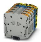
High-current terminal block, Blocked, Connection method: Power-Turn connection, Number of positions: 4, Cross section: 25 mm² - 95 mm², AWG: 4 - 3/0, Width: 100 mm, Color: gray/blue, Mounting type: NS 35/15
