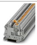
Knife disconnect terminal block, With test socket screws for insertion of test plugs, Connection type: Screw connection, Cross section: 0.2 mm² - 10 mm², AWG: 24 - 8, Nominal current: 20 A, Nominal voltage: 500 V, Length: 57.8 mm, Width: 8.2 mm, Color: gray, Assembly: NS 35/7,5, NS 35/15
