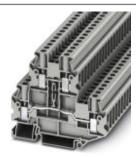
Double-level terminal block, Cross section: 0.14 mm² - 6 mm², AWG: 26 - 10, Connection type: Screw connection, Width: 6.2 mm, Color: gray, Mounting type: NS 35/7,5, NS 35/15
