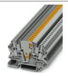
Test disconnect terminal block, With test socket screws for insertion of test plugs, Connection method: Screw connection, Cross section: 0.14 mm² - 6 mm², AWG: 26 - 10, Width: 6.2 mm, Color: gray, Mounting type: NS 35/7,5, NS 35/15
