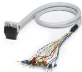
Round cable set with Single wires (14-position) (The wires are marked and fitted with ferrules.) on 1 x IDC/FLK socket strip (14-position, 90 °-Out put), Cable length: 3 m
