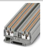
Feed-through terminal block, Connection method: Push-in connection, Cross section: 0.14 mm<sup>2</sup> - 4 mm<sup>2</sup>, AWG: 26 - 12, Width: 5.2 mm, Height: 35.3 mm, Color: white, Mounting type: NS 35/7,5, NS 35/15
