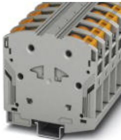
High-current terminal block, Connection method: Power-Turn connection, Cross section: 25 mm 2 - 95 mm 2 , AWG: 4 - 3/0, Width: 25 mm, Color: gray, Mounting type: NS 35/15
