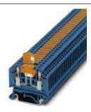
Knife disconnect terminal block, With test socket screws for insertion of test plugs, Connection type: Screw connection, Cross section: 0.2 mm² - 4 mm², AWG: 24 - 12, Nominal current: 16 A, Nominal voltage: 400 V, Length: 46 mm, Width: 5.2 mm, Color: blue, Assembly: NS 35/7,5, NS 35/15, NS 32
