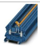
Knife disconnect terminal block, With test socket screws for insertion of test plugs, Connection type: Screw connection, Cross section: 0.14 mm² - 4 mm², AWG: 26 - 12, Nominal current: 20 A, Nominal voltage: 400 V, Length: 57.8 mm, Width: 5.2 mm, Color: blue, Assembly: NS 35/7,5, NS 35/15
