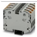
High-current terminal block, Connection method: Power-Turn connection, Cross section: 2.5 mm<sup>2</sup> - 35 mm<sup>2</sup>, AWG: 12 - 2, Width: 16 mm, Color: gray, Mounting type: NS 35/15
