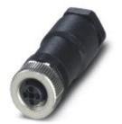
Connector, 4-position, Socket straight M12, T-coded, Screw connection, Knurl material: Zinc die-cast, nickelplated, Cable gland Pg9, External cable diameter 6 mm ... 8 mm, for direct current up to 12 A/60 V
