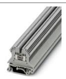
Feed-through terminal block, Connection method: Screw connection, Cross section: 0.14 mm² - 1.5 mm², AWG: 26 - 16, Width: 4.2 mm, Color: violet, Mounting type: NS 35/7,5, NS 35/15, NS 32
