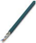
CAT5-SF/UTP cable (J-LI02YS(ST)C H 2 x 2 x 26 AWG), light-duty, flexible installation cable 2 x 2 x 0.14 mm<sup>2</sup>, stranded, shielded, outer sheath: 5.75 mm ± 0.15 mm diameter, preassembled on both sides with RJ45 plug, crossover or line assignment
