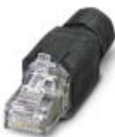
RJ45 connector, IP20, CAT5e, 8-pos., with QUICKON fast connection technology, for 1-wire and 7-wire conductors AWG 26 ... 22, for cable diameter of 4.5 mm ... 8.0 mm, TIA 568 B labeling, color: black
