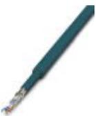
CAT5-SF/UTP cable (J-02YS(ST)C HP 2 x 2 x 24 AWG), heavy-duty installation cable, 2 x 2 x 0.22 mm<sup>2</sup>, solid conductor, shielded, outer sheath: 7.8 mm diameter, inner sheath: 5.75 mm ± 0.15 mm diameter
