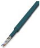
CAT5-SF/UTP cable (J-02YS(ST)C HP 2 x 2 x 24 AWG), heavy-duty installation cable, 2 x 2 x 0.22 mm<sup>2</sup>, solid conductor, shielded, outer sheath: 7.8 mm diameter, inner sheath: 5.75 mm ± 0.15 mm diameter, preassembled on both sides with RJ45 plug, crossover or line
