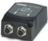
Passive network isolator with pre-installed adapter for mounting on a DIN rail. Electrical isolation in Ethernet networks. For protection against potential differences up to 4 kV. Transmission speed of up to 100 Mbps. M12 sockets (D-coded).
