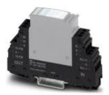
Base element to accept a protective plug with diagnostic and status indicator for two signal wires with common reference potential, integrated spark gap to provide a high-resistance connection between the ground of the protective circuit of the plug and ground potential.
