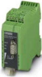
Fiber optic converter with integrated optical diagnostics, alarm contact, for PROFIBUS up to 12 Mbps, termination device with one fiber optic interface (SC-Duplex), 1300 nm, for fiberglass cable
