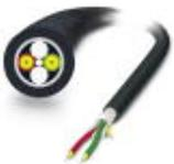
Highly rugged GOF round cable (IP20 heads only) for assembly and for outdoor installation with integrated moisture barrier as well as rodent-proof scrim. Individual elements made from highly flexible FRNC material. The wire is ozone and UV resistant with a very rugged polyethylene outer sheath.
