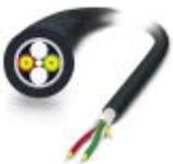
Highly rugged GOF round cable for assembly and for outdoor installation with integrated moisture barrier as well as rodent-proof scrim. Individual elements made from highly flexible FRNC material. The wire is ozone and UV resistant with a very rugged polyethylene outer sheath.
