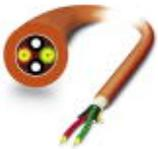
rugged GOF installation cable for inner areas with highly tear-proof aramid strain-relief elements. Individual elements consist of highly flexible FRNC material. The cable is halogen-free, ozone and UV resistant and has a rugged polyurethane (PUR) outer sheath.
