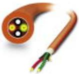
rugged GOF installation cable (IP20 heads only) for inner areas with highly tear-proof aramid strain-relief elements. Individual elements consist of highly flexible FRNC material. The cable is halogen-free, ozone and UV resistant and has a rugged polyurethane (PUR) outer sheath.
