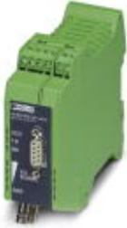
FO converter with integrated optical diagnostics, alarm contact, for PROFIBUS up to 12 Mbps, terminal equipment with an FO interface (BFOC), 850 nm, for fiber glass cable
