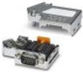
D-SUB connector, 9-pos., male connector, cable entry < 35°, bus system: PROFIBUS DP up to 12 Mbps, termination resistor can be switched on via slide switch, pin assignment: 3, 5, 6, 8; screw connection terminal blocks
