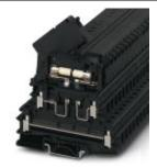
Fuse modular terminal block, Connection method: Screw connection, Cross section: 0.2 mm²- 4 mm², AWG: 24 - 12, Nominal current: 32 A, Nominal voltage: 400 V, Width: 8.2 mm, Fuse type: G / 6,3 x 32, Fuse type: Glass, Mounting type: NS 35/7,5, NS 35/15, NS 32, Color: black
