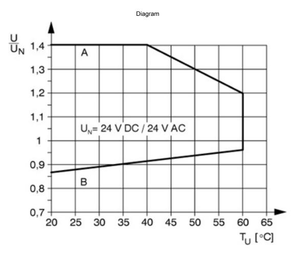
$\label{eq:curve} \mbox{Curve A} \\ \mbox{Maximum permissible continuous voltage $U_{max}$ with limiting continuous current on the contact side (see relevant technical data)}$
