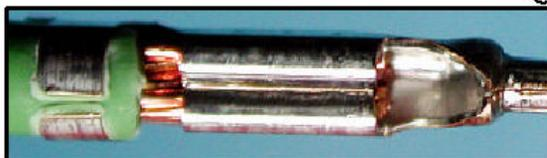
NO BOTTOM CORE WING FLARE ( PASSES PULL TEST )
