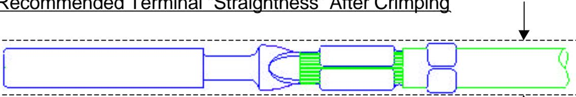
Terminal must fit a MAX. 2.10 Diameter
