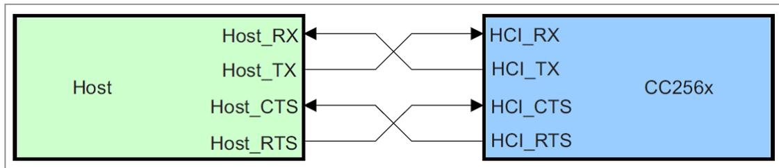
When the UART Rx buffer of the CC256x passes the “flow control” threshold, it will set the UART\_RTS signal high to stop transmission from the host.
