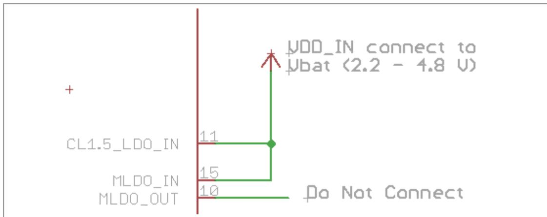
Full-DC2DC system (Lower RF output power, but optimum system power):
