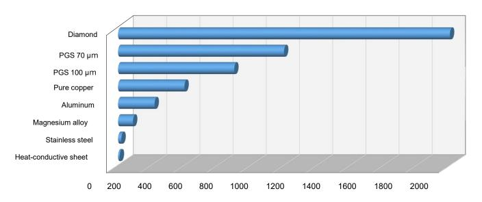
Coefficient of thermal conductivity W / (m·K)
