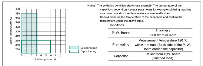
• The film capacitor has lower mounting heatresistingtemperature than other capacitors, therefore the following cautions are needed.
