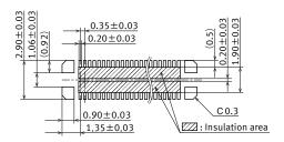
Recommended metal mask pattern Metal mask thickness: When 100µm (Terminal opening ratio: 85%) (Metal-part opening ratio: 50%)
