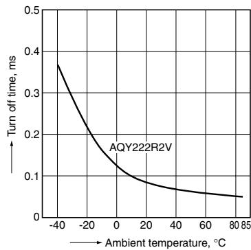
4.-(2) Turn off time vs. ambient temperature characteristics
