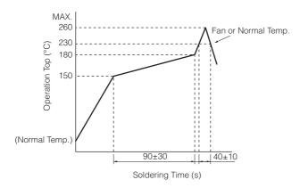
\* Reflow temperature may vary by location even in the same reflow condition. Please check the reflow temperature at terminals and at the top of a switch to make sure the both temperatures are withiin the specification. If even one of them is out of the specifications, please adjust.
