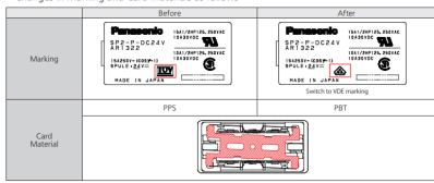
\*Although a representative example of the 2 Form C type is posted, 4 Form C type will be change in the same way.
